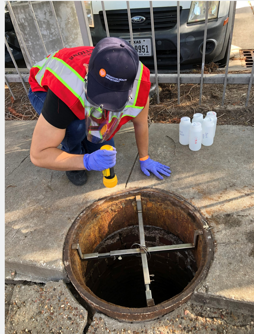
An environmental investigator from the Houston Health Department collects a sample from a manhole site in Houston, Texas.
